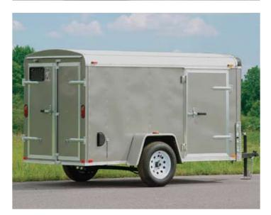
Atlas utility and cargo trailers begin with the same sturdy undercoated chassis and frame. Utility trailers have spring axles and bias tires, while the cargo trailers feature torsion axles and steel-belted tires. Of course, all trailers can be customized to fit your needs.
